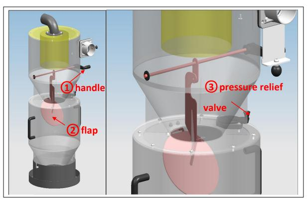
In normal working status, the flap is opening, the dust will drop down to the barrel below
