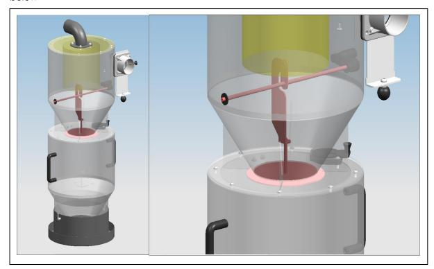
When changing bags, turning the handle ① to "Bag replacing" position, close the flap ②. Then open the pressure relief valve③, the dust in the barrel will drop down into the bags. Replace a new bag, while vacuum keeps working.
